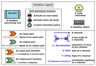
By convention, input ports are in orange, output ports in green, dataflow objects in light purple, dataflow units (e.g. processing or mock-up ones) are in light blue and comprise the symbol of their activation policy, and channels are in various shades of blue<sup>1</sup>.
