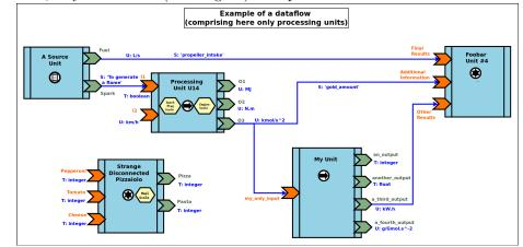
We can see that a dataflow does not need to be fully connected (the blocks may form disjoint subgraphs) and that ports (input and output ones alike) may not be connected either.
