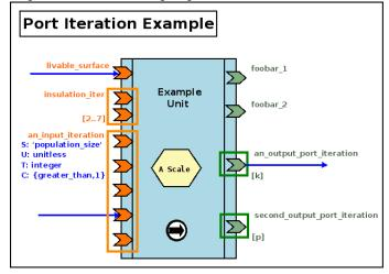
We can see above that, at any time, the first input iteration shall have between 2 and 7 (included) iterated ports, while the second input iterations is detailed graphically and has exactly 5 iterated ports ([5] is thus implied).
