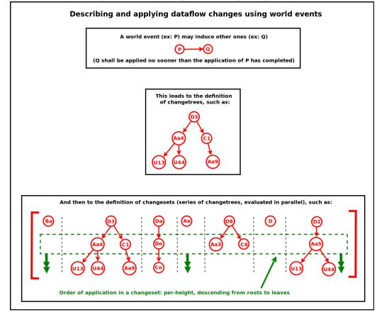
It is the role of the dataflow entry point (typically fetching its informations from an external source) to stream the corresponding changesets to the world manager, and to notify it when the synchronisation has been fully described (i.e. when all changesets have been transmitted).
