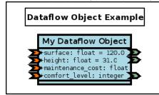
In this example, all attributes are standard, "bidirectional" attributes (they can be read and/or written by other dataflow blocks), except the maintenance cost, which is a "terminal" attribute (in the sense that it can be set, yet cannot be read by other blocks of the dataflow).
